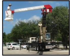
The CraneMate Phase Lifter Jib Boom pins to your crane's existing swing jib sheave head. The attachment design can transform many existing cranes (equipped with boom function radio remotes) into highly specialized insulated aerial lift bucket trucks. Excellent for delicate transmission line work; fiberglass basket optional.
