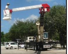
The *CraneMate Phase Lifter Jib Boom* pins to your crane's existing swing jib sheave head. The attachment design can transform many existing cranes (equipped with boom function radio remotes) into highly specialized insulated aerial lift bucket trucks. Excellent for delicate transmission line work; fiberglass basket optional.
