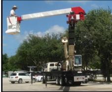
The *CraneMate Jib Boom* pins to your crane's existing swing jib sheave head. The attachment design can transform many existing cranes (equipped with boom function radio remotes) into highly specialized non-insulated aerial lift bucket trucks. Excellent for delicate cell tower maneuvers.
