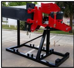
The patented *CraneMate<sup>TM</sup> Insul-Lift* jib boom pins to your crane's existing swing jib sheave head. The attachment design can transform many existing cranes (equipped with boom function radio remotes) into highly specialized insulated aerial lift bucket trucks.
